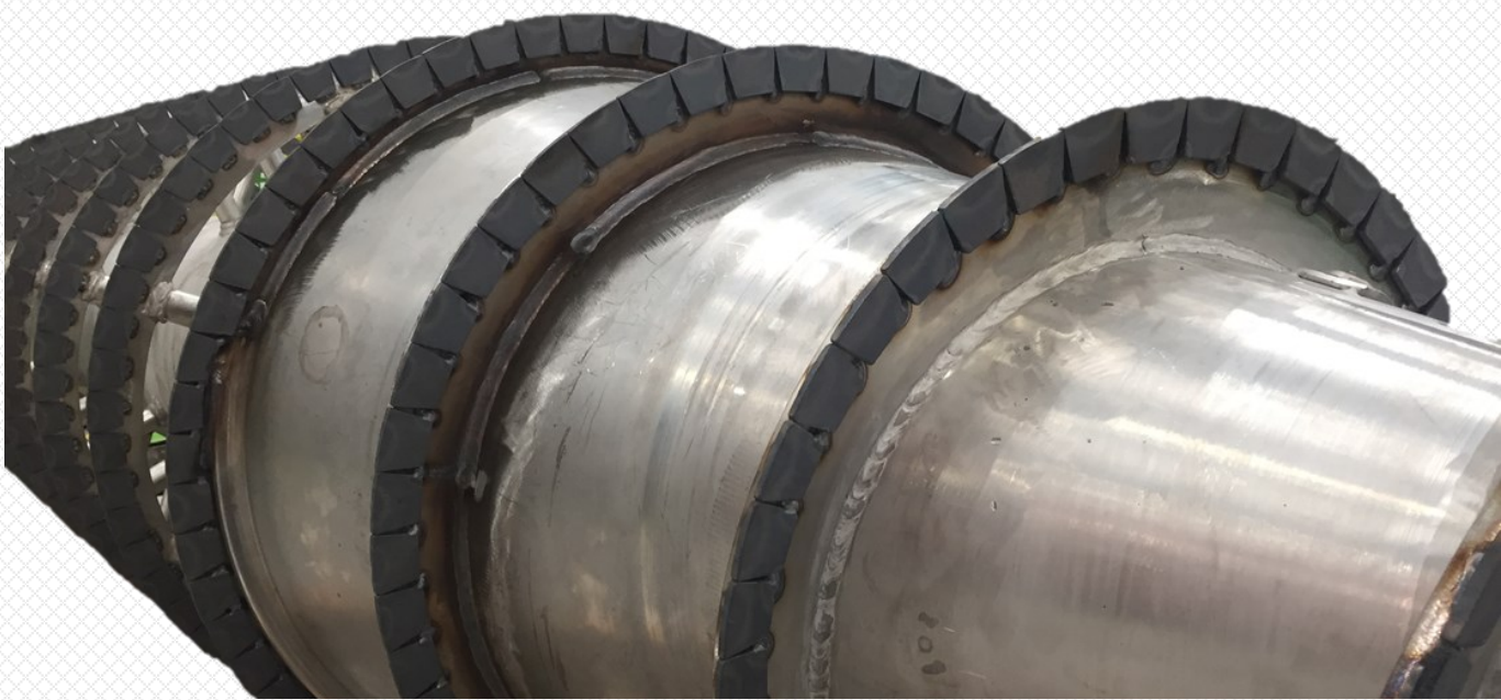
Decanter centrifuge fitted with Ferobide tiles, Courtesy of Brettex Site Services
